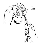
With your finger between the lines, wrap the lines evenly and firmly around the spool in a clockwise direction.
